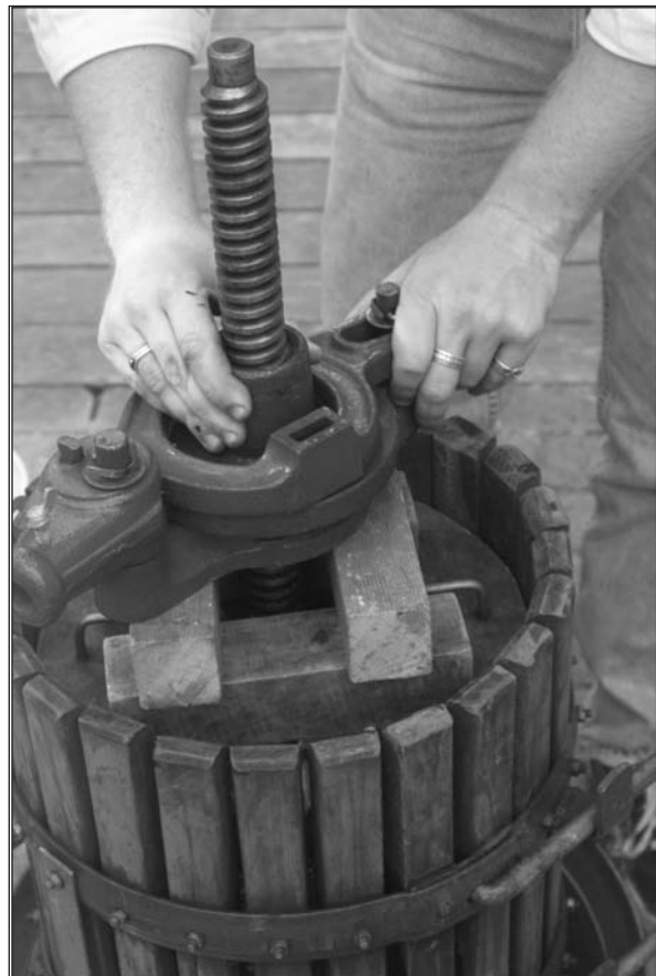
Placing the wood blocks and press head into the press before actually pressing the grapes.
