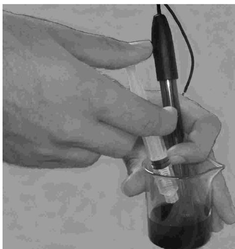
Figure 2. Manual stirring technique. Hold the electrode against the side of the vessel and swirl gently; add titrant with other hand.
