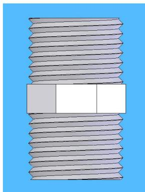
A common thread on European made wine equipment is BSPP (British Standard Pipe Parallel). BSPP threads are often called straight (parallel) threads. NPT and BSPP threads have different angles, shape, and (in most cases) threads per inch (pitch). The thread angle is 60° for NPT threads; 55° for BSPP threads.
