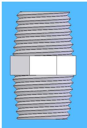
The standard thread found in the USA, and the default thread found on most all fittings in the MoreFlavor! Brands, is National Pipe Taper threads, abbreviated to NPT. NPT threaded fittings have a slight taper to them and when mated together and tightened, the threads compress to form a seal. Some confusion may result from the use of NPT, FPT, and MPT in describing threads.
